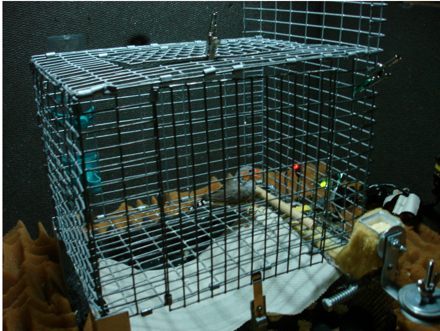
(a) The psychoacoustics setup consists of a cage which houses a perch and two LEDs, which are the observation and report keys. The food hopper (on the right) is brought up via a solenoid, and allows access to food through a hole in the floor of the cage.
